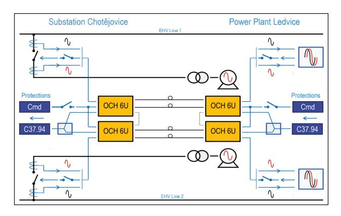
"Thanks to the unique capability of our device - 50 Hz phase transfer with the required maximum fidelity, the customer has solved the problem of a metallic cable failure, and at the same time gained an economical and secure solution for the transmission of distance and differential protection signals in one PCM30U-OCH"
