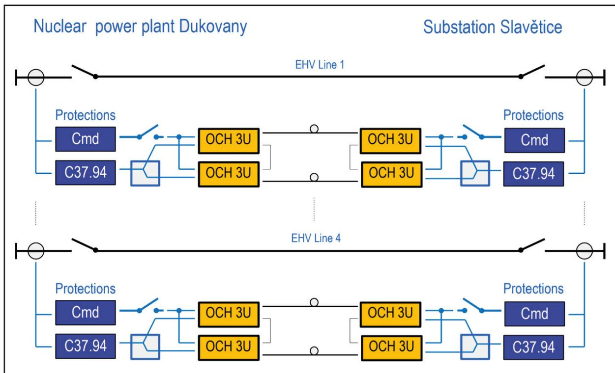
"Thanks to the installation of our PCM30UOCH, our customer has been able to quickly and efficiently transfer the necessary communication between the power station and the substation, including detailed monitoring of the status of transmission paths and devices, recording time and speed of transferred commands or database of failures," says Libor Jedlička, Project Manager of TTC Marconi.
